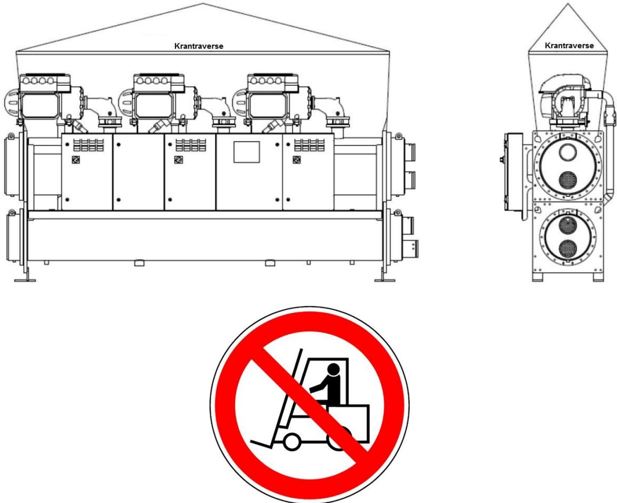
Figure 1. Transportation with crane at frameless design
