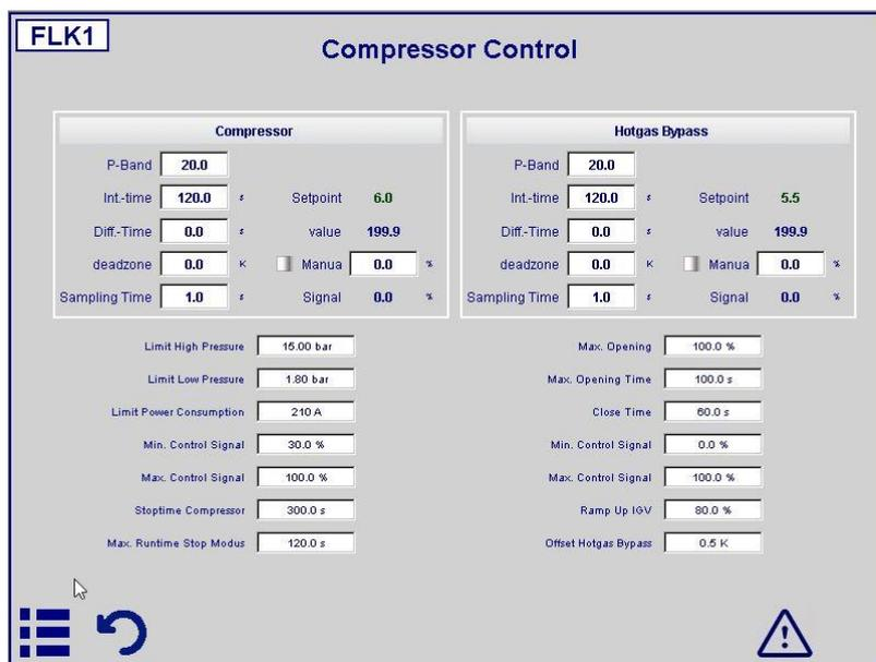
Figure 21. Compressor Control Menu
