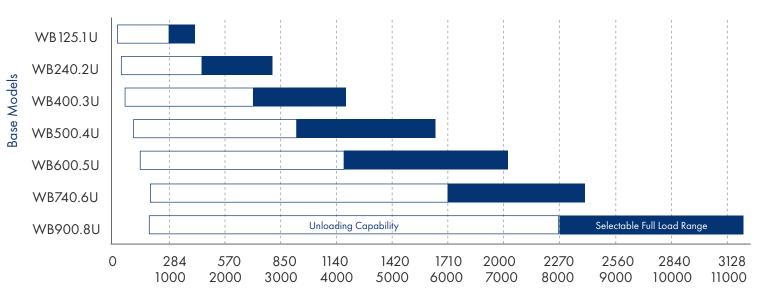
Cooling Capacity TR [kWR]
